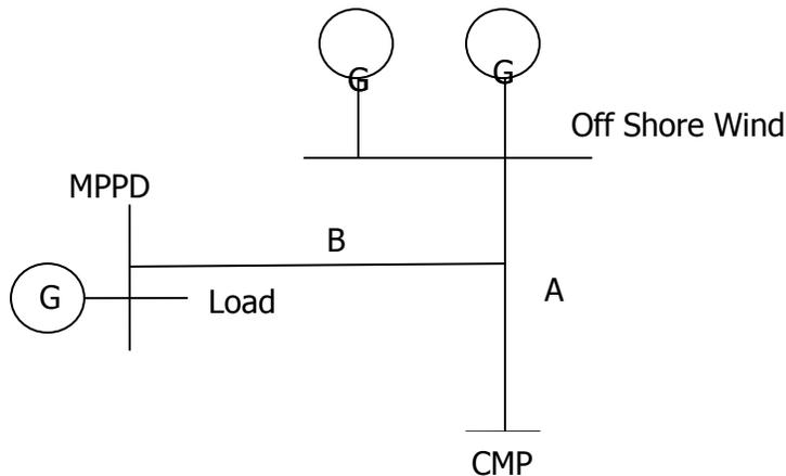
The Off Shore Wind project will connect to the on shore power system, owned and operated by Central Maine Power (CMP), via the subsea cable identified as "A". This will allow power to flow in both directions:
